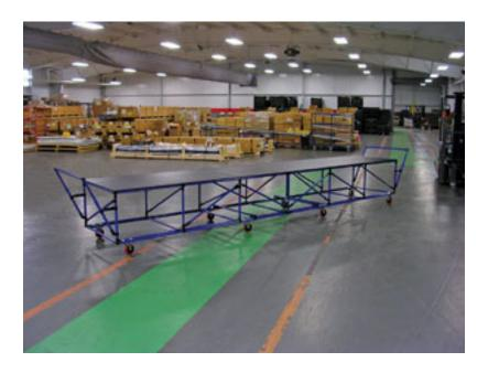
**Creform Corporation** (Greer, SC) has built the Extreme Size Car—which can be manufactured in virtually any size—to meet needs in large parts handling. The parts feature an elevated load platform with a solid plastic shelf surface to provide for damage-free handling of sensitive parts. Additional features include:
