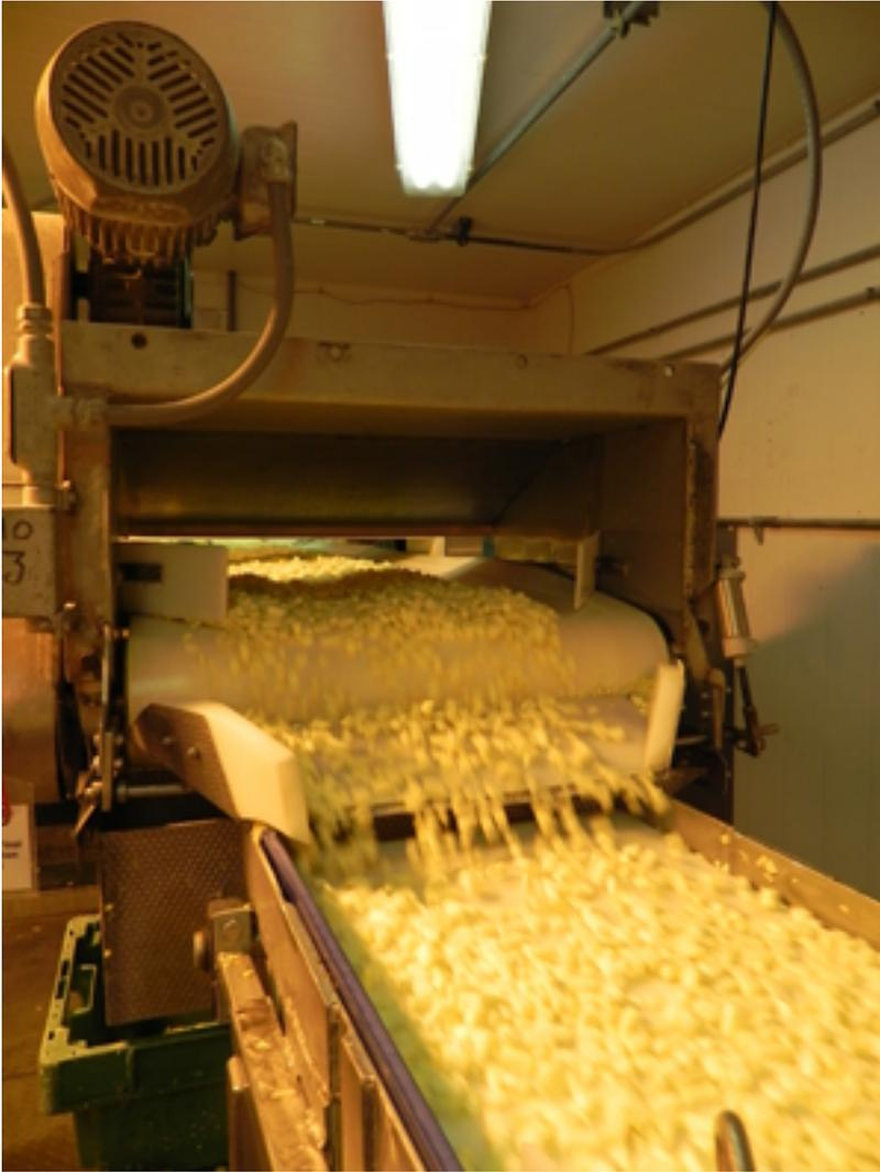
*Cleaned, peeled and cut apples are conveyed through a wash on their toward the fruit dryers.*
