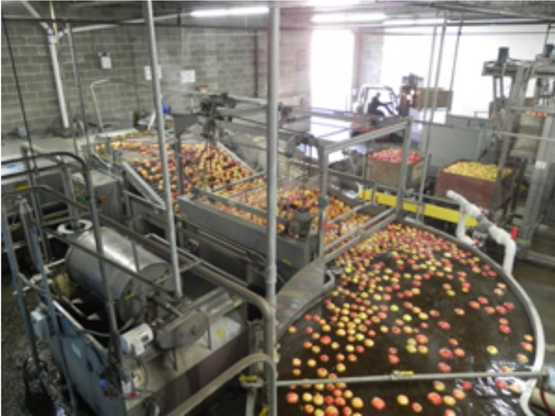
*Before being cleaned and peeled, apples are soaked to loosen any debris that may be on the fruits' surface.*
