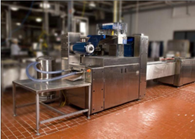
**Highly efficient, ultra-sanitary HFFS machine uses Rexroth integrated motor and drive, pneumatics, machine control and linear motion system.**
