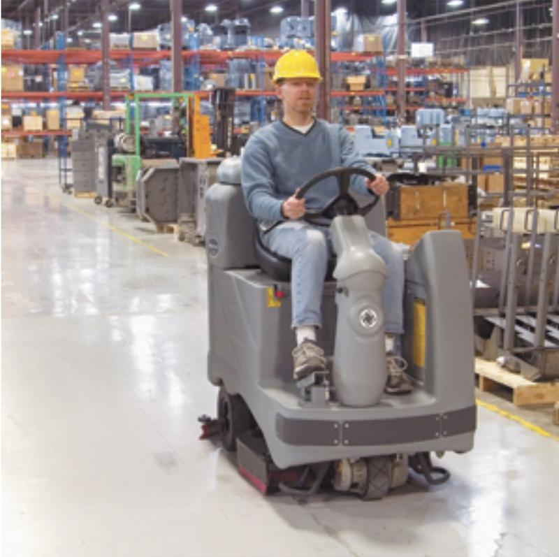
Floor scrubbers should be flexible enough to allow the operator to choose where to apply extra water or detergent, such as in higher-traffic or spill areas.
