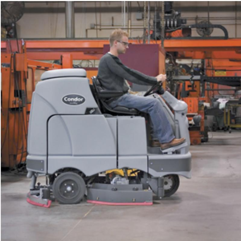
Newer floor-cleaning machines can be big water-savers because they use ultra-low-flow dispensing that cuts water usage by up to 70 percent.
