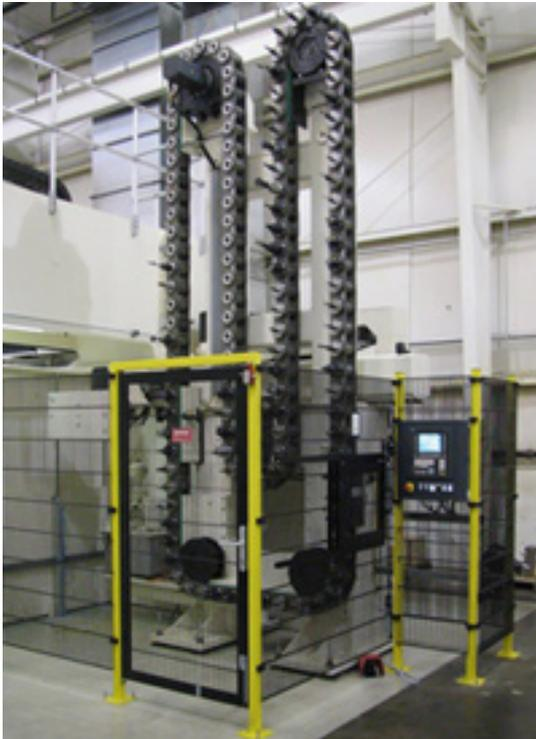
120-position tool carriage holds various HSK63 and HSK100 tooling.
