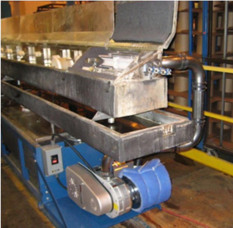
When it comes to fenestration, the components of today's energy efficient doors and windows should be made with the same attention to resource management. Recently the Amesbury Group's Textile Facility, part of its Sealing Solutions Division, completed a compressed air reduction project which will yield a \$41,000 annual electricity cost savings in their extrusion department. Yet, replacing compressed air nozzles with a blower-powered air wipe system wasn't as simple as it first appeared.
