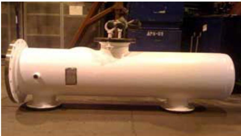
New heat exchanger shell that was fabricated by APS for a process line at a leading national brewery. The white coating is an epoxy that helps to reduce corrosion.
