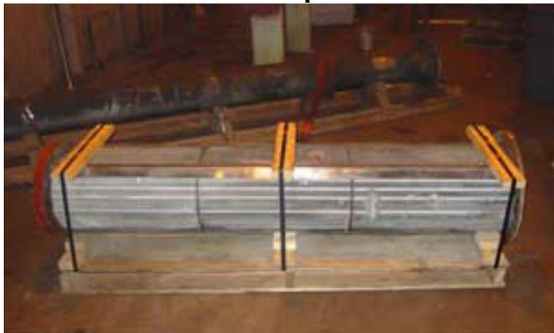
Process Heat Exchanger Tube Bundle Rebuilt by American Power Services
