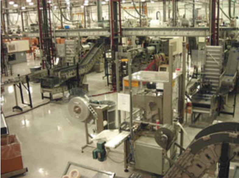
Traditionally, conveyors are sensitive pieces of equipment needed frequent alignment, belt replacement, and lubrication. Because reconfigurable modular conveyors are maintenance-free, engineering departments are free to hang the systems without worry about taking down conveyors to work on them.
