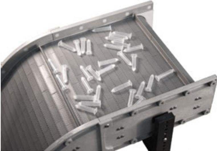
With modular conveyor systems, changes are made by swapping out modules with the release of a few bolts and snapping the modules in or out. Because the belt is also modular in design, links can easily be changed with the release of a few pins.
