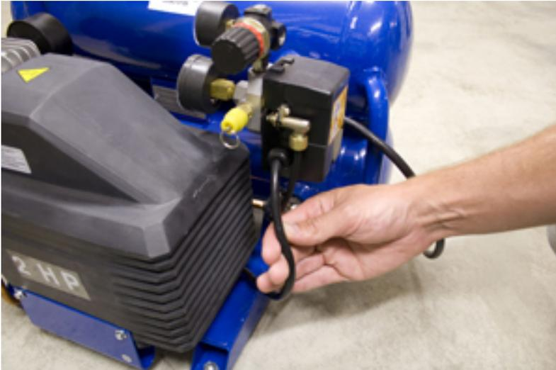
Check the hoses for kinks, the electrical wiring for cuts and fraying, and the tubing and piping for any damage.
