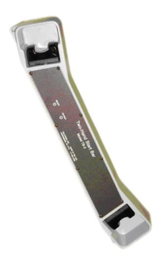
Featuring optic sensors that require no force to actuate, the model TB-2 Start Bar reduces fatigue and injuries caused by repeatedly pressing a mechanical start switch. The angle and spacing of the sensors coincide with the natural motion of the operator's hands, reducing hand and wrist stress.
