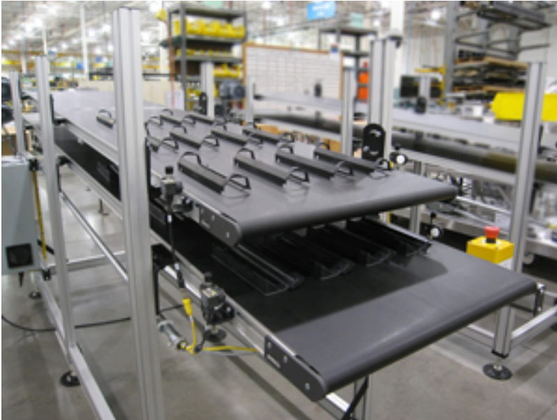
Dorner's two-tier conveying system.
