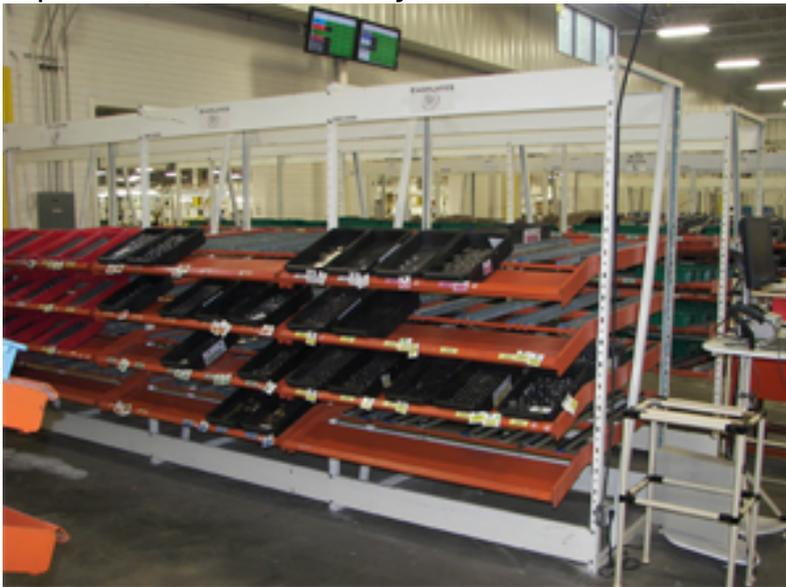
The implementation of this Kanban system for machined parts helped to greatly improve the inventory levels and on-time delivery rates of **Snap-on's Murphy, NC** power tool plant.
