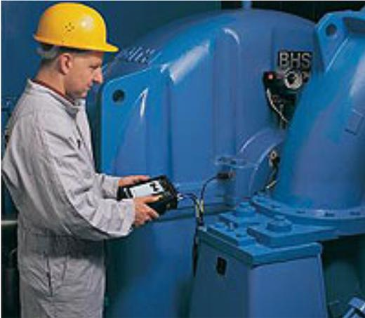
**Utilizing** a data collector/vibration analyzer can help you diagnose machine health. (Photo credit: Ludeca)
