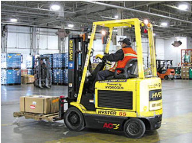
**Hydrogenics and LiftOne** join forces to power a forklift with a hydrogen fuel cell. The vehicle should be able to refuel in minutes, as opposed to the hours it would take to recharge a battery.
