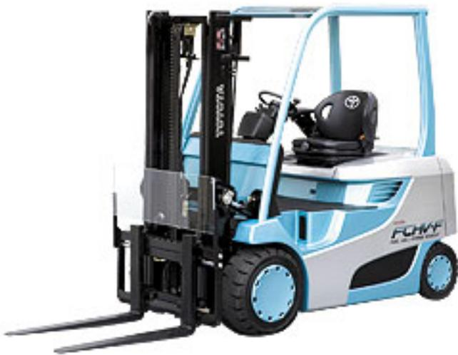
**Toyota's prototype FCHV-F** generates zero carbon dioxide emissions, and should be available within the next several years.
